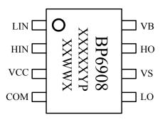
Figure 2. Pin configuration
